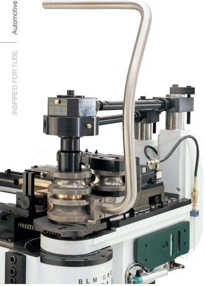
The introduction of CNC technology to tube bending represents a step change in the way in which tube is manipulated, and the BLM Dynamic fiveaxis tube bending machine recently installed in Toolspec Manufacturing's Luton factory is very much a case in point.
